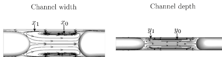
Figure 3: Illustration of the recirculation inside the liquid slug in microfluidic reactor at Taylor flow (adaptation of Abadie et al. 2013 29 ).
