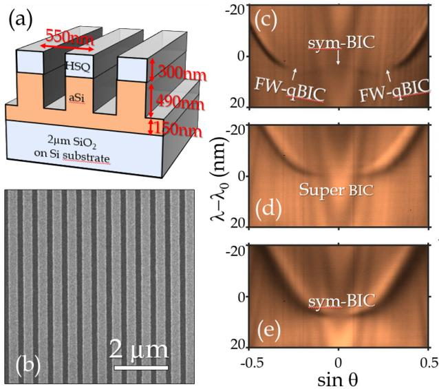
FIG. 4. (a) Sketch of the sample design. (b) SEM image of a grating structure (here  $f = 0.39$ ). (c-e) Angle-resolved reflectivity measurements of three structures having three different filling factors  $f$  that correspond to (c) before merging, (d) at the merging transition, (e) after the merging transition. To follow the same photonic band, the spectral range of 40 nm is centred at  $\lambda_0 =$  (a) 1043 nm, (b) 1020 nm, (c) 1007 nm.
