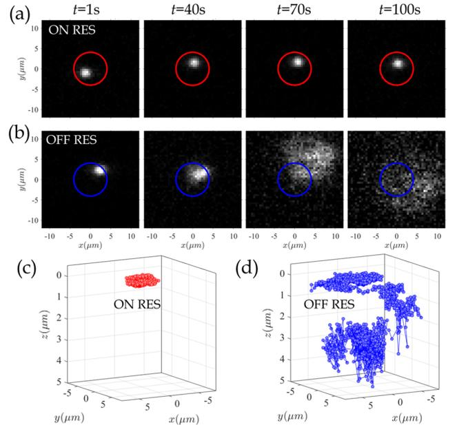
FIG. 5. (a,b) Frames captured when the laser is on resonance (a), then off resonance (b) with the super BIC. The red (blue) circle corresponds to the laser spot at on (off) resonance with the super BIC. (c,d) Coordinates of the particles extracted from the captured frames when the laser is on resonance (c), then off resonance (d) with the super BIC.
