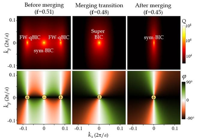
FIG. 3. (First row) Quality factor of the upper band as a function of  $k_x$  and  $k_y$ . (Second row) Orientation angle  $\varphi$  of the far-field polarization of the upper band. These results are obtained by using the analytical model based on the Friedrich-Wintgen formalism (1).
