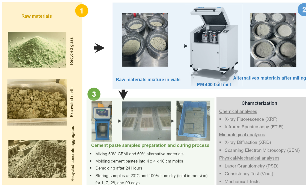
Figure 1. Schematic representation of the steps from raw materials to the preparation of alternative materials and the manufacturing of cement pastes and modified cement paste samples.
