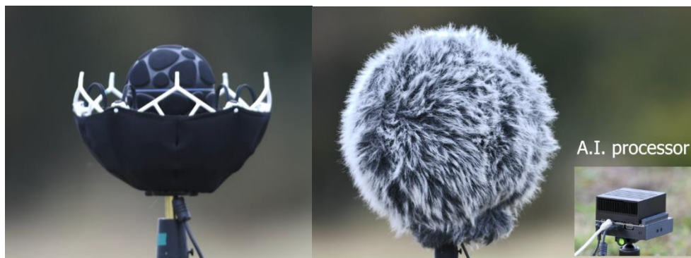
Figure 1: View of the 19 MEMS microphone antenna without (left) and with (right) environmental protection, and Nvidia Jetson associated with the antenna.
