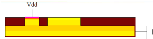
Fig.4: 2D TCAD structure used for the extraction of the N-well which corresponds to the R_{cnpn} of the compact bipolar transistor model.
