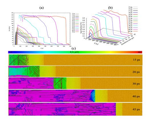
Figure 8: : Spatial profiles of the longitudinal pressure  $P_z$  (a) and hcp phase fraction (b) along the wave propagation axis z for a defective [001]-oriented single crystal iron when the bcc to phase is highly over-compressed to a piston maximum velocity of 1600  $m.s^{-1}$  during 30 ps. (c) selected snapshots of atomic configuration showing the wave propagation, defects associated with the plastic deformation and local phase structures. The atoms colors are the same as in Fig. 2.
