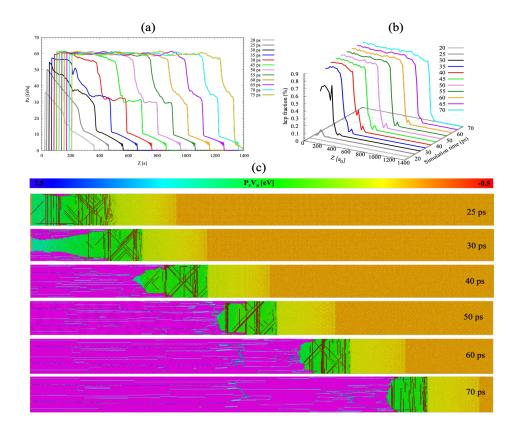
Figure 6: : Spatial profiles of the longitudinal pressure  $P_z$  (a) and hcp phase fraction (b) along the wave propagation axis z for a defective [001]-oriented single crystal iron when the bcc to phase is overcompressed to a piston maximum velocity of 1000  $m.s^{-1}$  during 30 ps. (c) selected snapshots of atomic configuration showing the wave propagation, defects associated with the plastic deformation and local phase structures. The atoms colors are the same as in Fig. 2.
