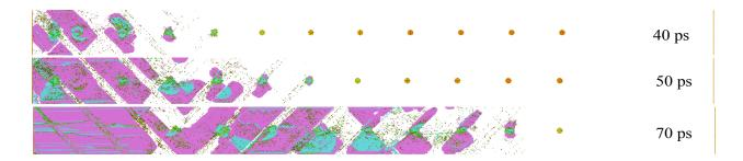
Figure 3: Nucleation and growth of the high pressure hcp phase (violet colored atoms), including some atoms of fcc type (cyan colored atoms), around the initial defects in a defective single crystal iron ramp-compressed to a piston maximum velocity of 600  $m.s^{-1}$  (same as Fig. 2d, but without displaying the bcc atoms).
