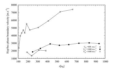
Figure 4: bcc/hcp phase boundary velocity for maximum piston velocities of 600  $m.s^{-1}$  (a), 1000  $m.s^{-1}$  (b) and 1600  $m.s^{-1}$  (c). In this latter case, the phase boundary progressively accelerates during its propagation and overtakes the longitudinal sound speed of about 6  $km.s^{-1}$  in iron.
