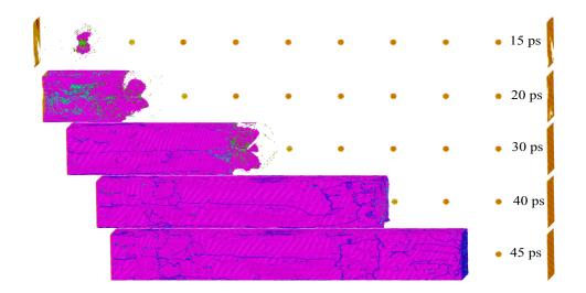
Figure 9: Nucleation and growth of the high pressure hcp phase (violet colored atoms), including some atoms of fcc type (cyan colored atoms), around the initial defects in a defective single crystal iron where the bcc to hcp phase transition is highly over-compressed to a piston maximum velocity of 1600  $m.s^{-1}$  (same as Fig. 8 without displaying bcc atoms).
