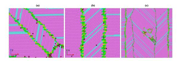
Figure 5: : Atomic configurations in y-z (a) and x-z (b) sections showing the microstructure in the hcp phase with primary twins (region between the two lines of green-colored atoms) issued from the plastic activity in the bcc phase. (c) cross-section perpendicular to the z-axis across the twin of (b) showing secondary twinning activity resulting from the hcp phase nucleation and growth.
