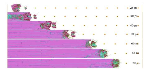
Figure 7: : Nucleation and growth of the high pressure hcp phase (violet colored atoms), including some atoms of fcc type (cyan colored atoms), around the initial defects in a defective single crystal iron when the bcc to hcp phase transition is over-compressed to a piston maximum velocity of 1000  $m.s^{-1}$  (same as Fig. 6c, but without displaying the bcc atoms).
