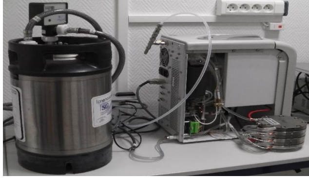
Figure 1. Investigated PEM electrolyzer system for education purposes
