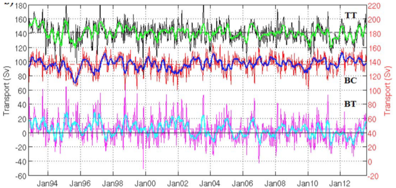
Figure 2: Time series of the total (in black), baroclinic (in red), and barotropic (in magenta) transport from 0 to bottom, with their smoothed time series (respectively green, blue, and light blue) obtained with a 1 month running mean. Total mean: 141 Sv, std: 13 Sv. Barotropic mean: 5 Sv, std: 16 Sv. Baroclinic mean: 136 Sv; std: 11 Sv. Note that the red right axis to the right refers to the baroclinic transport only.
