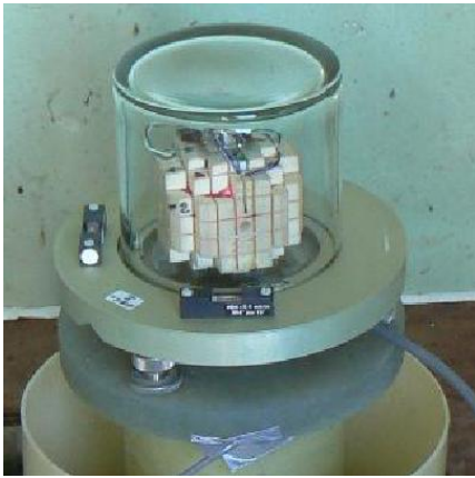
Figure 1: The IGP VM391 tri-axis fluxgate magnetometer.
