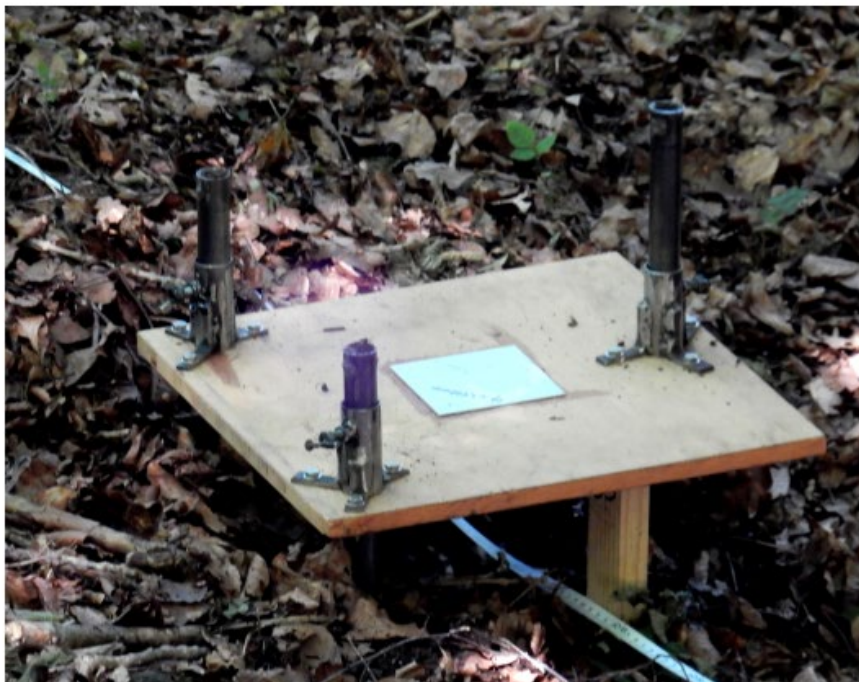
182 Fig. 6. Design and photo of the first platform installed. It consists of three sliding feet that 183 move vertically thanks to three vertical guides. The sliding tubes are locked with screws once 184 the mobile posts are in place. The wooden platform is levelled thanks to a level indicator, so 185 that the levelling of the gravimeter requires a minimum and residual work. This system can 186 cope with high slopes despite loose ground, while the posts can be driven 10 to 40 cm deep.
