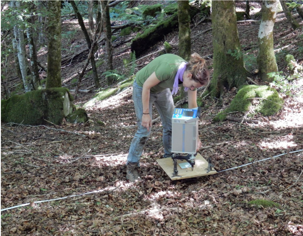
173 Fig. 5. This picture shows the ground conditions. The gravimeter is leveled using the 174 Gravimeter 3 micrometer screw system, but a special plywood platform has been designed 175 to make the instrument easier to set up. Without this, levelling would have been extremely 176 difficult, if not impossible. This platform is shown in detail in Fig. 6.
