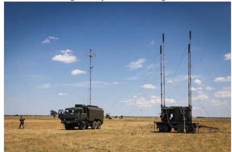
A Russian R-330ZH Zhitel station used to jam GPS signals
