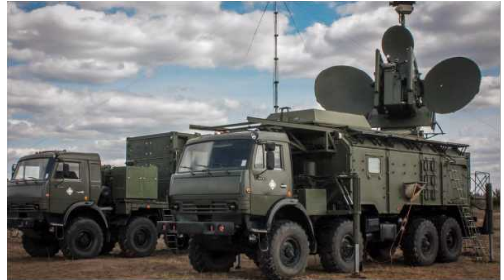
A Russian Krasukha-4 jamming station was captured in Ukraine in March The Russian Krasukha-4 is designed to jam low-orbit signals, drones and missiles
