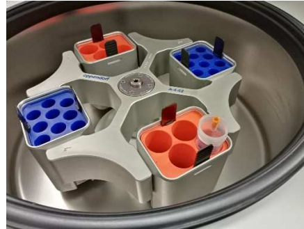
Figure 3. Image of the centrifuge used in the experimental campaign. Only the 2 orange swing buckets were used, in order
