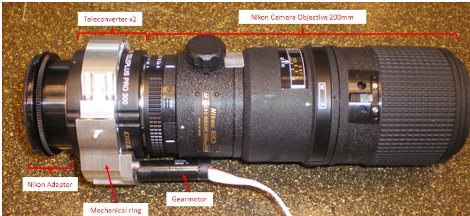
Figure 6: General view of camera objective {Nikon Adaptor + Teleconverter x2 + Motorization + Camera Objective}
