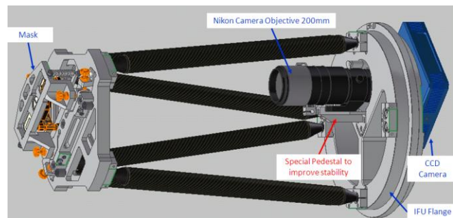
Figure 12: Mechanical drawing of the special pedestal
