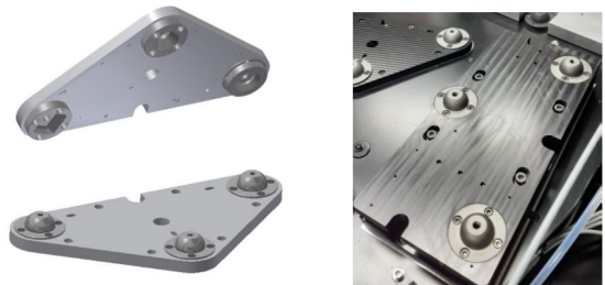
Figure 5: Left: Foreseen adjustments to reach requirements. Right: Kinematic mounting based in PLP
