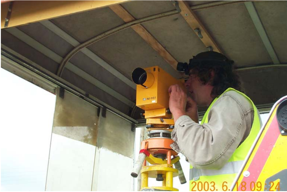
Figure 7: Surveyor operating a Zeiss NI002 level for scientific levelling.
