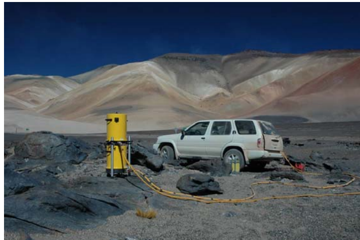
Figure 6: The new portable absolute gravity meter (A10#014) in field operation (north Chile).
