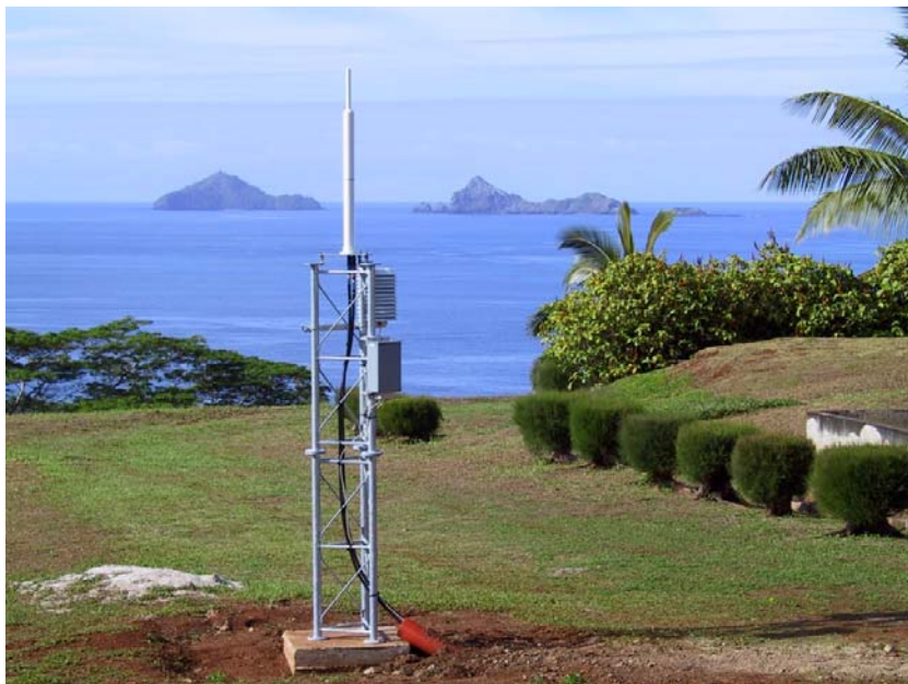
Figure 1: DORIS permanent tracking station in Rikitea (French Polynesia). From H. Fagard (IGN/SIMB).
