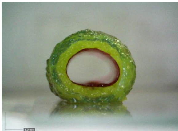
Figure 9. Three layered vascular construct obtained using extrusion based approach on a rotating cylinder
