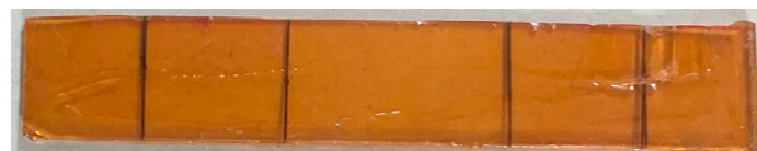
Figure 2. DGEBA/CA/cardanol vitrimer polymer specimen.
