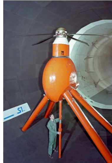
Figure 1: ERATO setup in ONERA’s S1MA wind tunnel.
