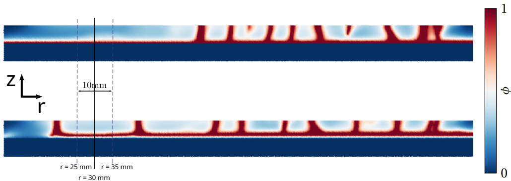
Fig. 12 Result of phase-field nodal variable \phi for detached nodes (top) and attached nodes (bottom)
