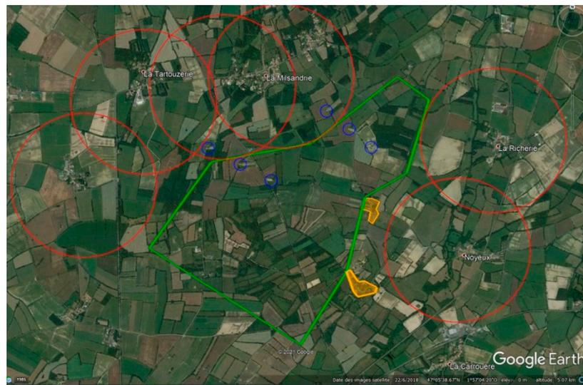
**Figure 4.** The authorized flight area is delimited with the green line. The small blue circles are the wind turbines. The red circles border the populated zones. The three wind sectors (WSs) are shown in green, peach, and pink (see text for more details).
