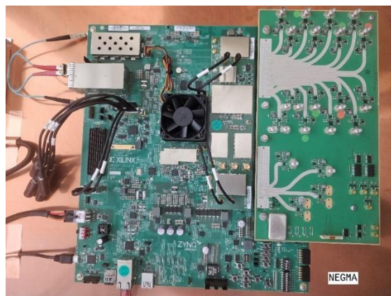
Figure 61: ZCU216 evaluation kit with a front-end board for input signals
