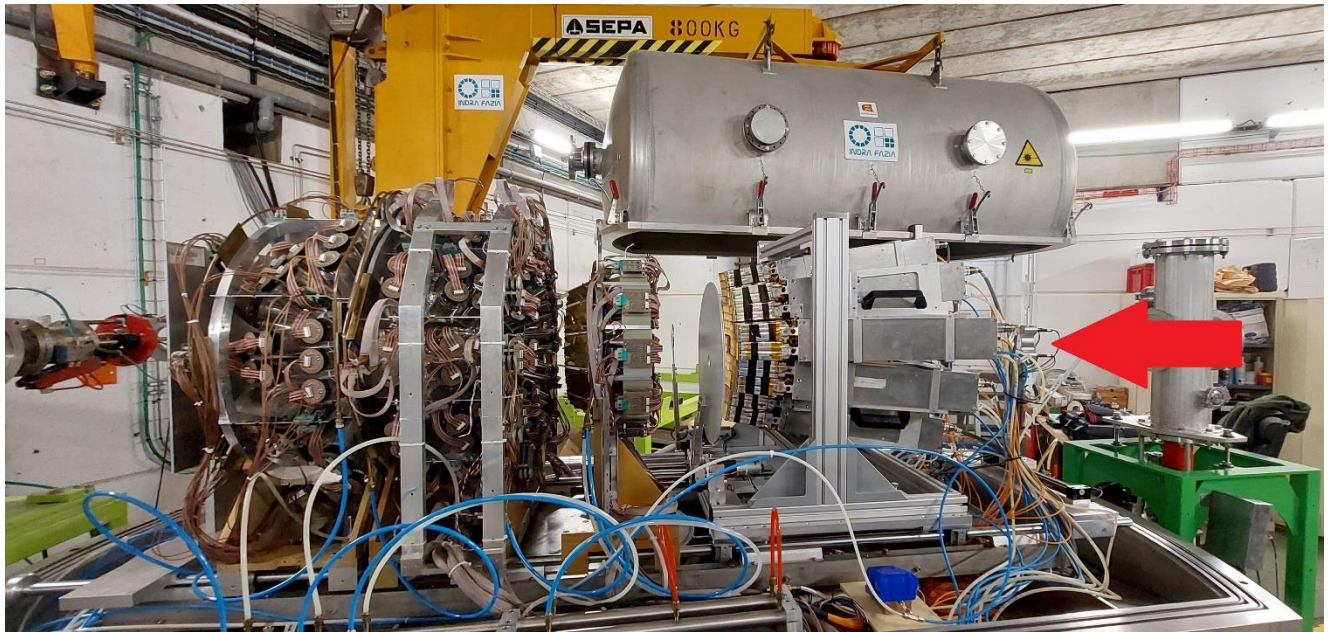
Figure 60 : INDRA (left)-FAZIA (right) apparatus in D5 at GANIL, the red arrow indicates the location of the beam detectors monitor downstream the beam line, behind the 12 FAZIA blocks.
