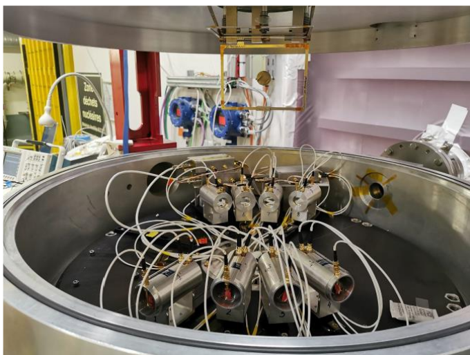
Figure 18: The MEDLEY detector with its 8 telescopes
