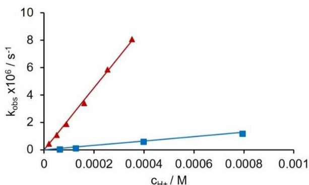
**Figure 4.** Dependence of the pseudo-first order dissociation rate constants on the acid concentration in Cu-transmetallation experiments for **CeL2** ( $\blacktriangle$ ) and **GdL2** ( $\blacksquare$ ). **CeL2**: pH 3.45 - 4.73,  $c_{\text{CeL2}} = 0.15$  mM,  $c_{\text{Cu}^{2+}} = 4.5$  mM; **GdL2**: pH 3.1-4.2,  $c_{\text{GdL2}} = 1$  mM,  $c_{\text{Cu}^{2+}} = 10$  mM 25 °C; I = 0.15 M NaCl.
