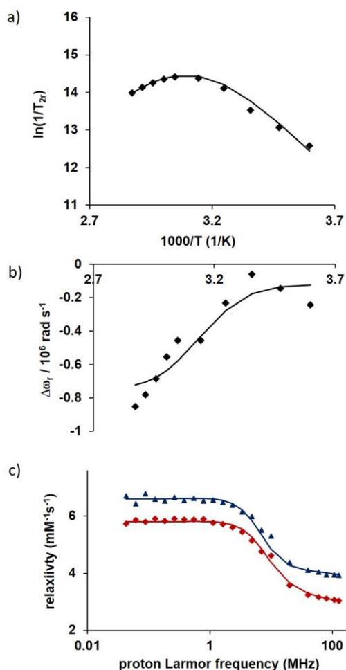
**Figure 5.**  $^{17}\text{O}$  transverse relaxation rates (a),  $^{17}\text{O}$  chemical shifts (b) (9.4 T,  $c_{\text{GdL2}} = 17.7$  mmol/kg), and NMRD profiles (1.79 mM) at 25 °C ( $\blacktriangle$ ) and 37 °C ( $\blacklozenge$ ) (c) measured for **GdL2**. The solid lines represent the simultaneous fit to all data as explained in the text.
