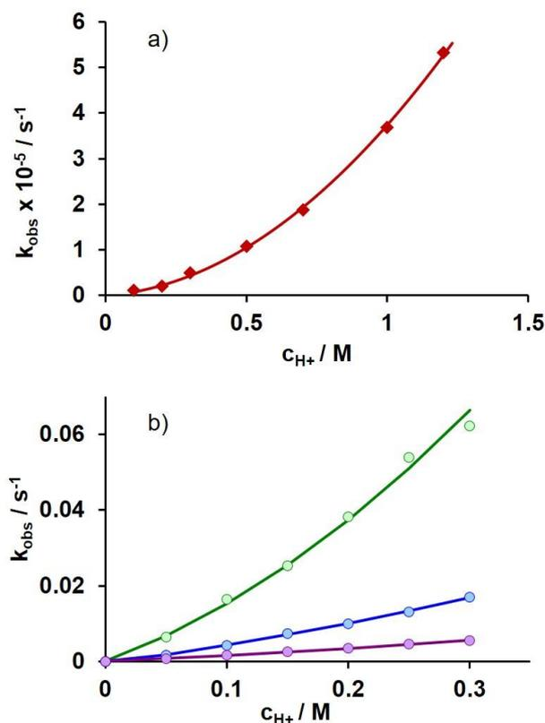
**Figure 3.** Dependence of the pseudo-first order dissociation rate constants on the acid concentration in highly acidic conditions for a) **GdL1** and b) **CeL2** (●; 0.225 mM); **GdL2** (●; 0.247 mM) and **YbL2** (●; 0.251 mM) complexes; 25 °C; I = 1 M NaCl. The lines correspond to the fit of the experimental data.
