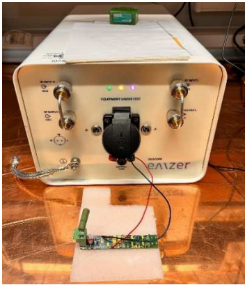
Fig. 13. EMC measurement setup using EMScope device.
