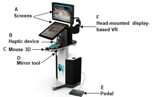
Figure 1 Haptic simulator VirTeaSy Dental® consists of various components: A) Screens connected to computer featuring touch interface for visualizing three-dimensional (3D) images. B) Haptic arm or physical handpiece enabling tactile interactions with simulator, providing real-time force feedback information. C) 3D mouse for controlling and interacting with simulator interface. D) Physical mirror linked to virtual mirror to facilitate visualization of dental procedures. E) Pedal for performing procedures, used to activate rotary instruments or other functions. F) Optionally, a virtual reality (VR) headset for full immersion in virtual environment.
