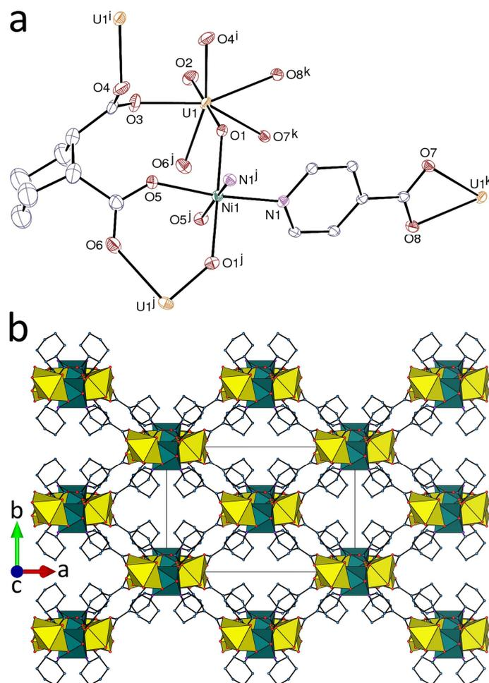
**Figure 1.** (a) View of complex **1**. Displacement ellipsoids are drawn at the 30% probability level. The solvent molecule and hydrogen atoms are omitted. Symmetry codes:  $i = 1 - x, 1 - y, 1 - z$ ;  $j = 1 - x, y, 3/2 - z$ ;  $k = 1/2 - x, 1/2 - y, 1 - z$ . (b) View of the triperiodic framework with uranium coordination polyhedra yellow and those of nickel(II) green.
