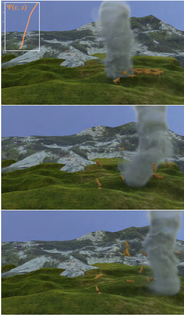
Figure 12: Rough terrain: The no-penetration boundary condition imposed by the reflected filament keeps the tornado nearly orthogonal even when the terrain is fairly uneven.
