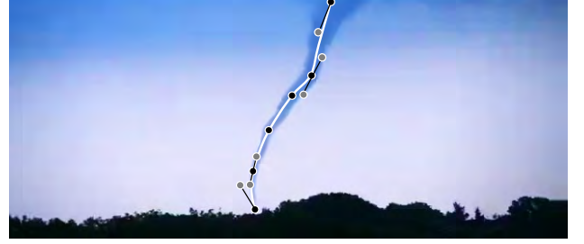
Figure 4: Core initialization: The user can specify the geometry of the core by placing and editing spline control points, e.g., fitting the spatial orientation of an existing tornado.
