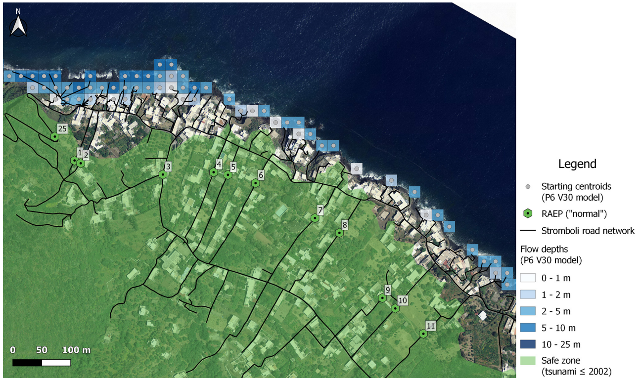
Figure 2. Establishment of baseline data: starting centroids for the numerical simulation of a 30 \times 10^6 \text{ m}^3 tsunamigenic landslide that detached from position number 6 (294 m b.s.l.) with a density of volcanic materials of 2.5 \text{ kg m}^{-3} and the Stromboli road network and refuge area entry points used to run evacuation models. The map was produced by the authors using Quantum GIS version 3.16.7 software (2021). Image data © 2014 LGS.
