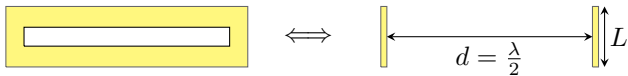
Fig. 3. Equivalent model of the loop resonator. The loop is replaced by two small dipoles spaced \lambda/2 apart with \lambda taken at the fundamental resonance frequency of the loop f_1 .
