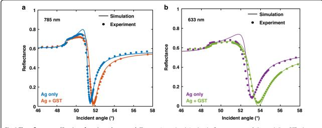
Fig. 2 The reflectance calibration of sensing substrate. a, b The experimental and simulated reflectance curves of silver and silver-GST substrates at 785 nm (a) and 633 nm (b)
