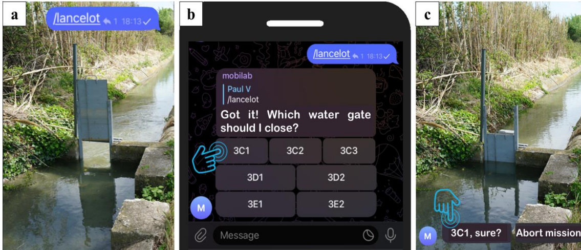
Figure 7. Operational « Lancelot » prototype in use during the 2023 irrigation season : a) surface irrigation gate in open position; b) the gate to be operated is selected by the farmer via the messaging interface ; c) the selected irrigation gate is remotely closed after user validation.
