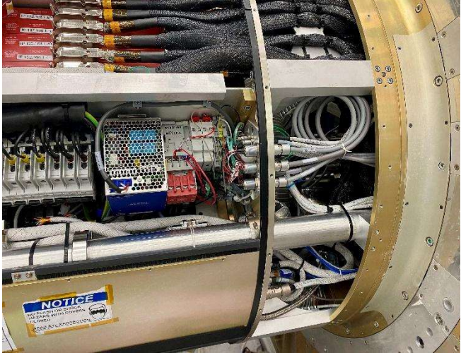
Figure 47: Utility trunk with outer skins removed
