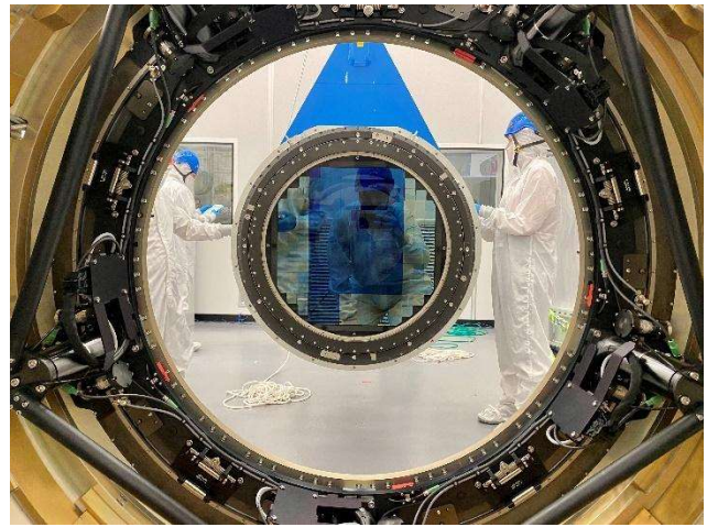
Figure 27: Cryostat being inserted into the camera body. Cover is removed from L3.
