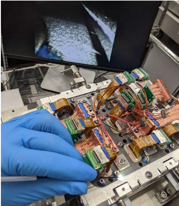
Figure 44: Verifying cleanliness on raft sensor assembly (RSA)
