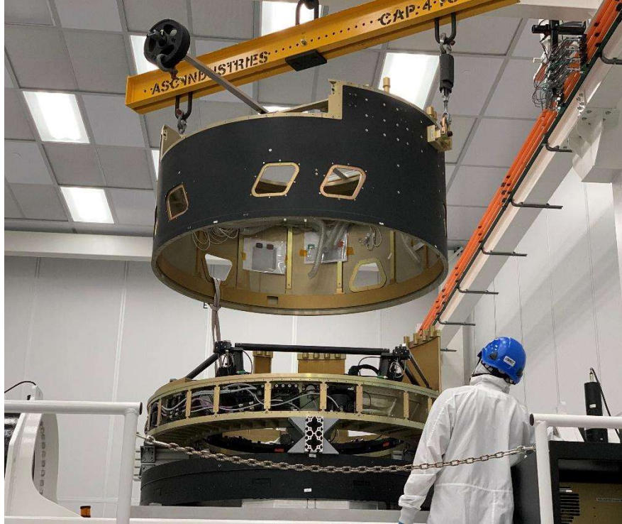
Figure 25: Camera housing (in black) integration with back flange (in gold). Part of the filter exchange system carousel is visible on the back flange.
