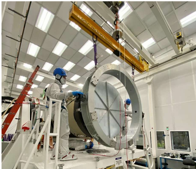
Figure 33: Removing the L1-L2 Lifting Ring from the Camera
