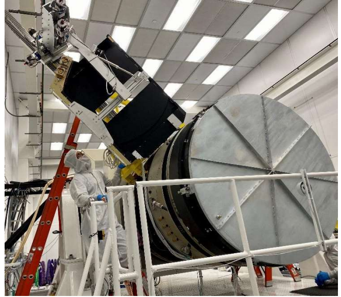
Figure 37: Shutter installed onto extraction rail
