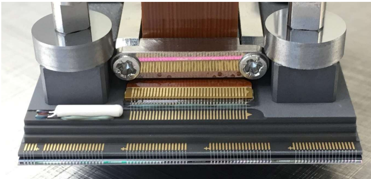
Figure 43: Example CCD with no metallic particles on wire bonds
