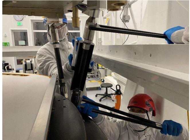
Figure 35: Adjusting the differential screw of the L1-L2 strut
