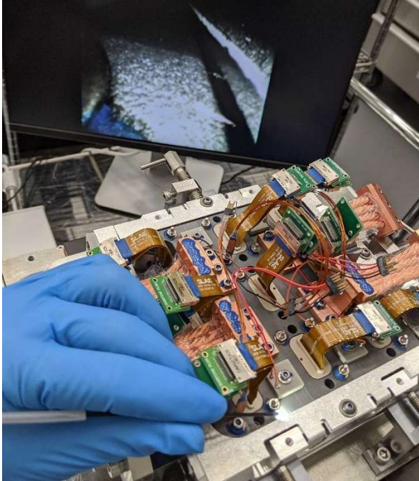
Figure 44: Verifying cleanliness on raft sensor assembly (RSA)
