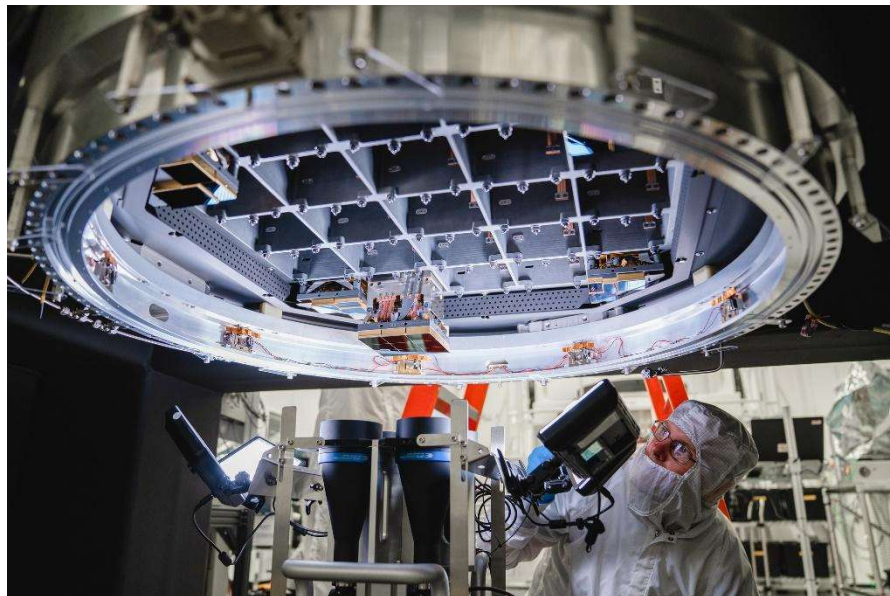
Figure 13: Cameras and lights installed to monitor the 4 corners of the raft assembly during installation. Credit: Jacqueline Orrell
