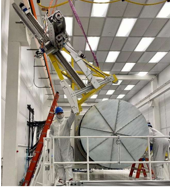
Figure 36: Shutter extraction rail lifted into place and bolted to outside diameter of camera body
