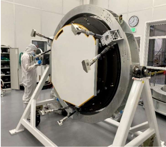
Figure 31: L1-L2 mounted to support stand which allows change in orientation
