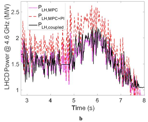
**Figure 13.** (a) Safety factor on the magnetic axis,  $q_0(t)$ , from real-time EFIT magnetic equilibrium reconstruction (solid) and  $q_{0,target}(t)$  (dashed red) in EAST discharge #94832. Control starts at  $t = 2.7$  s. (b) Coupled LH2 power (solid black) and MPC command before (dotted magenta) and after (dashed red) the PI actuator control in EAST discharge #94832. The coupled power (solid) closely matches the original controller command (dotted magenta). Control starts at  $t = 2.7$  s.
