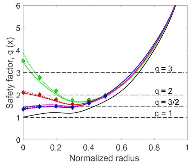
**Figure 10.** Simultaneous  $q_0$  and fast  $\beta_{\text{p}}$  control with LHCD and ICRH. Achieved profiles at  $t = 3.2$  s (black), 5 s (magenta), 9 s (red), 13 s (blue), and 18 s (green). The  $q(x)$  targets (diamond symbols) are held constant between these times, which are depicted by vertical lines on figure 9. Both  $q(x)$  and  $\beta_{\text{p}}$  control start at 3.2 s. The dotted lines are from distributed  $q(x)$  control and fast  $\beta_{\text{p}}$  control, for comparison.
