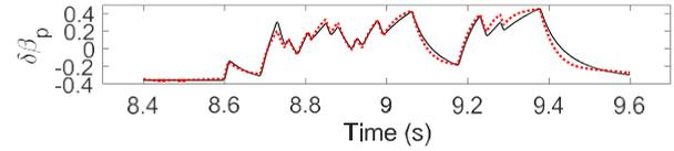
**Figure 4.** Comparison between the reduced  $\delta\beta_p$  data from METIS (black) and the ARTAEMIS-simulated data (red dotted) for high frequency ICRH power modulations. The corresponding input data are shown on figure 1 and the fit parameter for  $\delta\beta_p$  in this simulation is  $f = 83\%$ .
