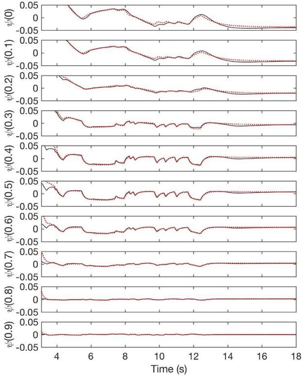
**Figure 2.** Comparison between the reduced  $\psi(x)$  data (Wb) at  $x = 0, 0.1, \dots, 0.9$  from METIS (black) and the ARTAEMIS-simulated data (red dotted) from the two-time-scale model for the simulation with low frequency modulations whose input data are shown on figure 1. In this simulation, the global fit parameter for  $\psi(x)$ , integrated from  $x_1 = 0$  to  $x_2 = 1$ , is  $f = 77\%$ .
