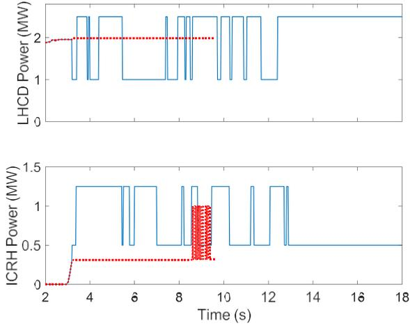
**Figure 1.** LHCD (top) and ICRH (bottom) power waveforms (MW) used in METIS simulations with low frequency modulations (blue) and high frequency modulations (red dotted).
