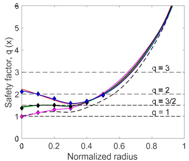
**Figure 12.** Simultaneous distributed  $q(x)$  and fast  $\beta_p$  control with LHCD and ICRH, and with  $\mu(x) = 1$  for  $0 \leq x \leq 0.5$ . Control of  $q(x)$  starts at 3.2 s while  $\beta_p$  control starts at 4.2 s. Achieved  $q(x)$  at  $t = 3.2$  s (dashed black), 9 s (magenta), 13 s (red), 17 s (blue), 21 s (green), and 25 s (solid black). The  $q(x)$  targets (diamond symbols) are held constant between these times, which are depicted by vertical lines on figure 11.
