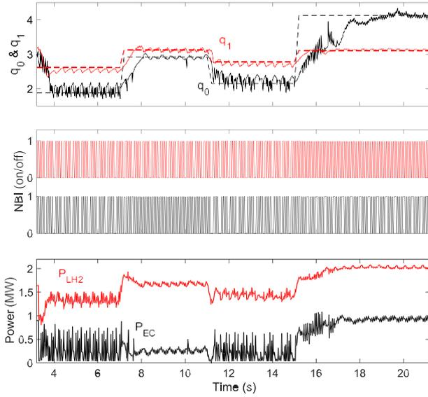
**Figure 15.** Simultaneous control of  $q_0$  and  $q_1 = q(x = 0.4)$  with LHCD, ECRH and NBI. Top frame:  $q_0$  (solid black trace),  $q_{0,target}$  (black dashed),  $q_1$  (solid red trace) and  $q_{1,target}$  (red dashed) vs time. Middle frame: NB1 (bottom, black) and NB2 (top, red) PWM (0 = off, 1 = on). Bottom frame: LH2 (red) and ECRH (black) actuator powers.
