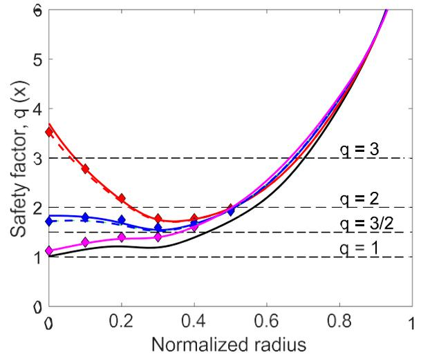
**Figure 6.** Distributed  $q(x)$  control with  $\mu(x) = 1$  for  $0 \leq x \leq 0.5$  and with LHCD only. Achieved  $q(x)$  at  $t = 3.2$  s (black),  $7.1$  s (magenta),  $13.1$  s (red solid), and  $18$  s (blue solid). Target  $q$ -profiles are constant during these intervals (diamond symbols). Dashed lines are profiles achieved with  $q_0$  control only (see figure 1).
