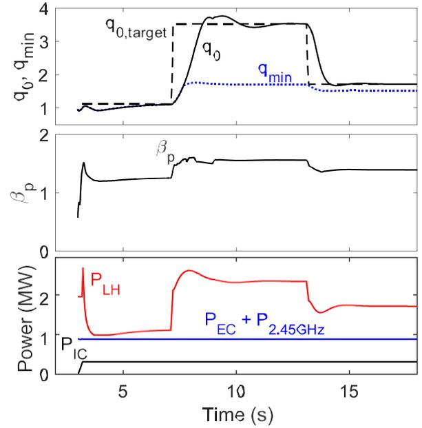
**Figure 5.** Control of  $q_0$  with LHCD. Top:  $q_0(t)$  (solid black),  $q_{0,\text{target}}(t)$  (dashed) and  $q_{\text{min}}(t)$  (dotted blue) vs time. Middle:  $\beta_p$  vs time (not controlled). Bottom: 4.6 GHz LHCD actuator power (red) and feedforward powers: ICRH (black) and combined ECRH plus 2.45 GHz LHCD (blue). Control starts at  $t = 3.2$  s.
