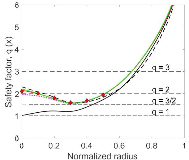
**Figure 8.** Combined distributed  $q(x)$  control and slow  $\beta_p$  control with LHCD and ICRH. Achieved  $q(x)$  at  $t = 3.2$  s (solid black), 5.1 s (dotted), 7.1 s (red), 9.1 s (blue), 10 s (dashed black) and 12.5 s (green). These times are depicted on figure 3 by vertical lines. The target  $q$ -profile is constant (diamond symbols) and  $\mu(x) = 1$  for  $0 \leq x \leq 0.5$ .  $q(x)$  control starts at 3.2 s while  $\beta_p$  control starts at 4.2 s.
