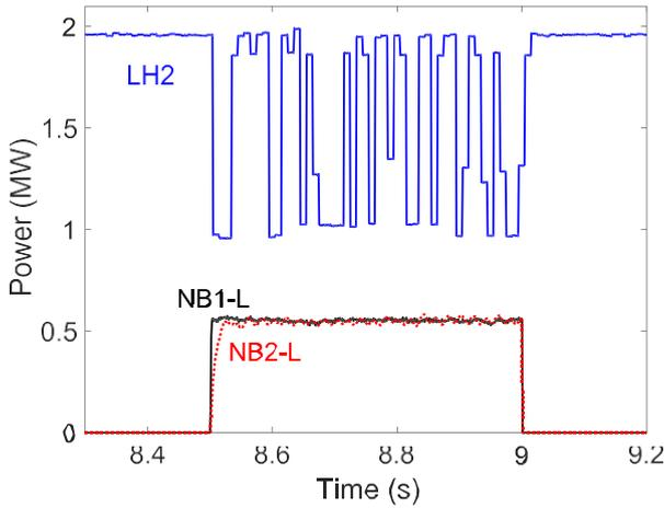
**Figure 18.** Fast LH2 power modulations (blue trace) injected from PRBS commands on discharge #126963. NB1-L (solid black trace) and NB2-L (dotted red trace) powers are also shown. The NB-R actuator is off.
