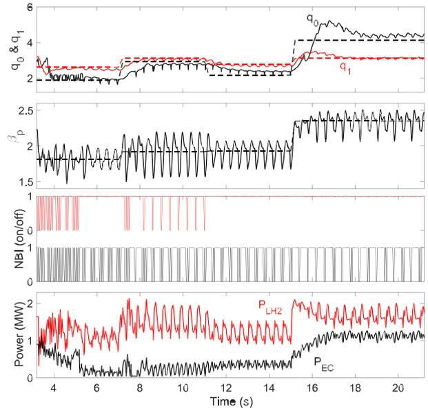
**Figure 16.** Simultaneous control of  $q_0$ ,  $q_1 = q(x = 0.4)$  and  $\beta_p$  with LHCD, ECRH and NBI. Top frame:  $q_0$  (solid black trace),  $q_{0,target}$  (black dashed),  $q_1$  (solid red trace) and  $q_{1,target}$  (red dashed) vs time. Second frame:  $\beta_p$  (solid black trace),  $\beta_{p,target}$  (black dashed). Third frame: NB1 (bottom, black) and NB2 (top, red) PWM (0 = off, 1 = on). Bottom frame: LH2 (red) and ECRH (black) actuator powers.
