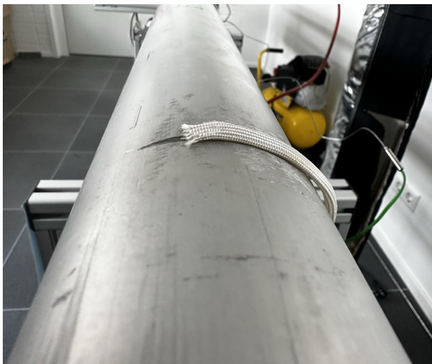
Fig. 5 Thermocouple attached to the aluminum shell in the ASTER. The thermocouples are placed within a heat resistant fabric sheath to prevent damage to the heating blankets
