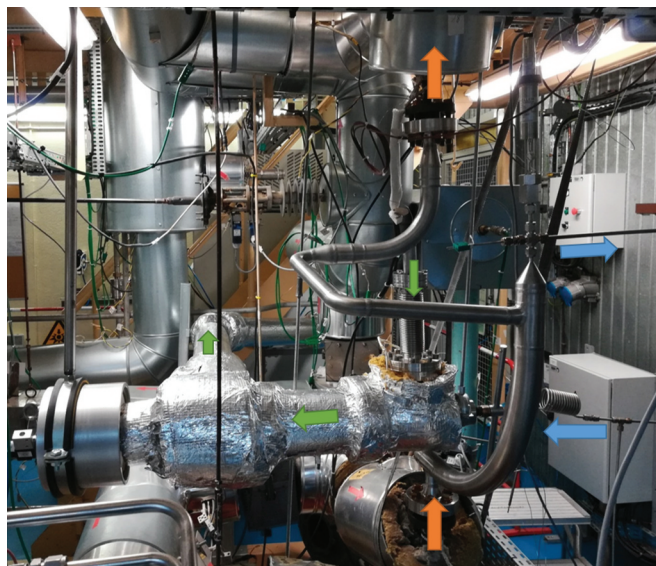
Fig. A.2. Picture of the TS: sodium circuit (orange arrows), gas circuit (blue arrows), and vacuum line (green arrows).
