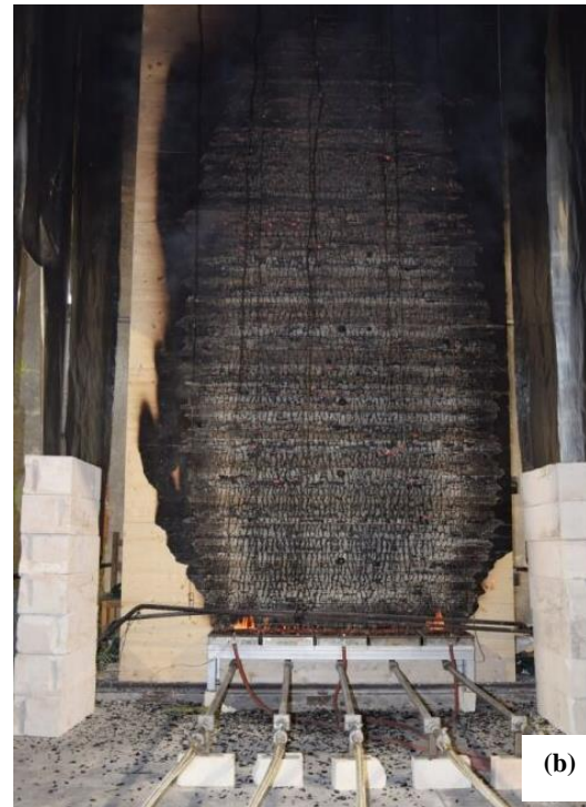
Figure 8 (a) picture after test (b) char depth distribution
