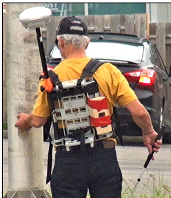
Fig. 2. The mobile GPS receiver carried by one of the participants in this study.
