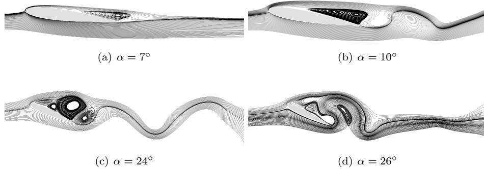
FIGURE 5. Streamlines around NACA 0012 for various angles
