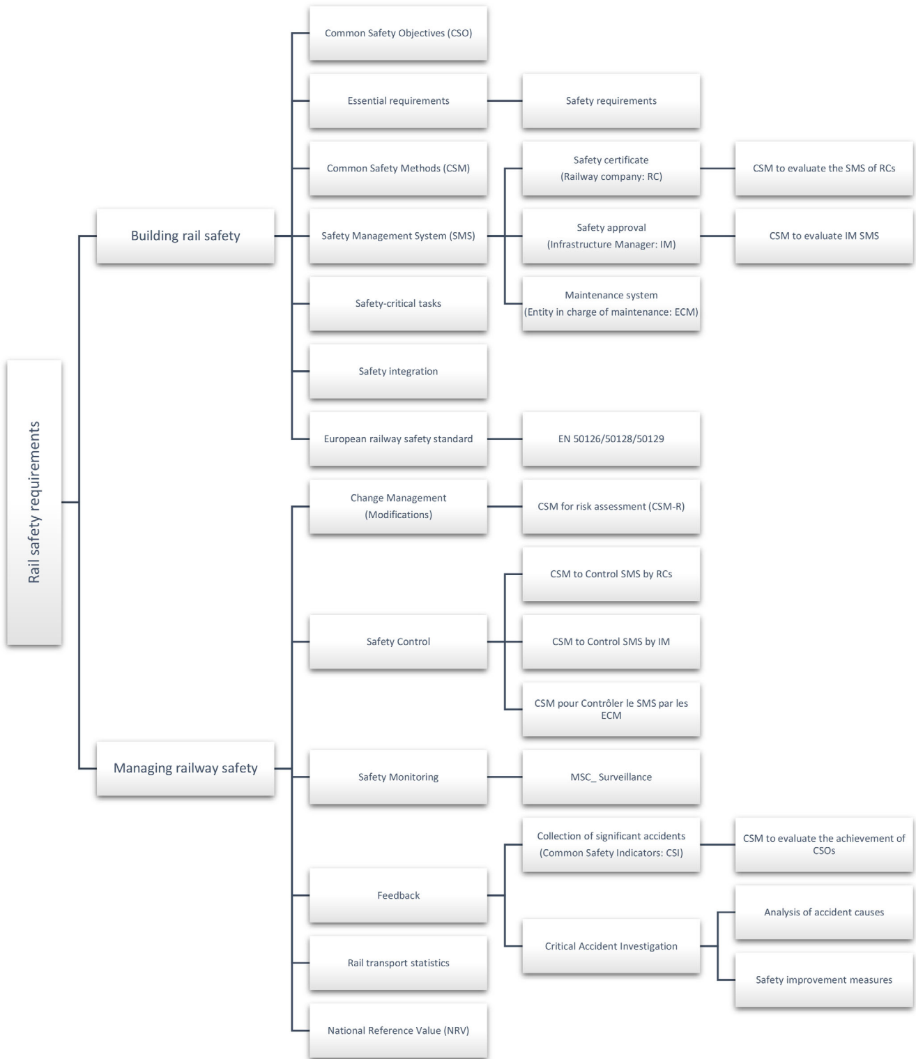
FIGURE 4 Main safety requirements according to the railway safety directive.
