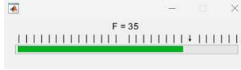
Fig. 4. Visual cue in the form of loading bar that increases with the pressing force (in gramme “gf”). The arrow represent the limit that should not be surpassed.
