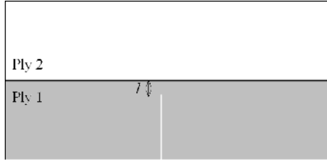
Fig. 10.13. A crack growing in Material 1 and approaching the interface, at a distance l .
