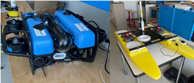
Fig. 2. ROV (Bluerov2) and USV (Hydrone-based) of the system.
