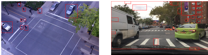
(a) Fixed camera with background subtractor. (b) Mobile camera with background subtractor.
