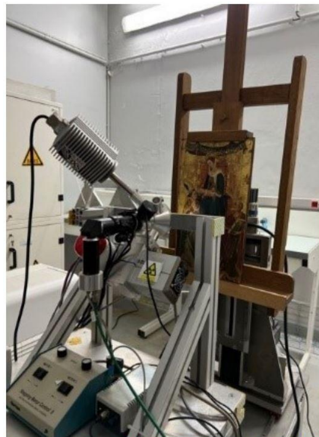
Fig. 2 CXRF prototype LouX 3D used with the painting at the C2RMF, Paris
