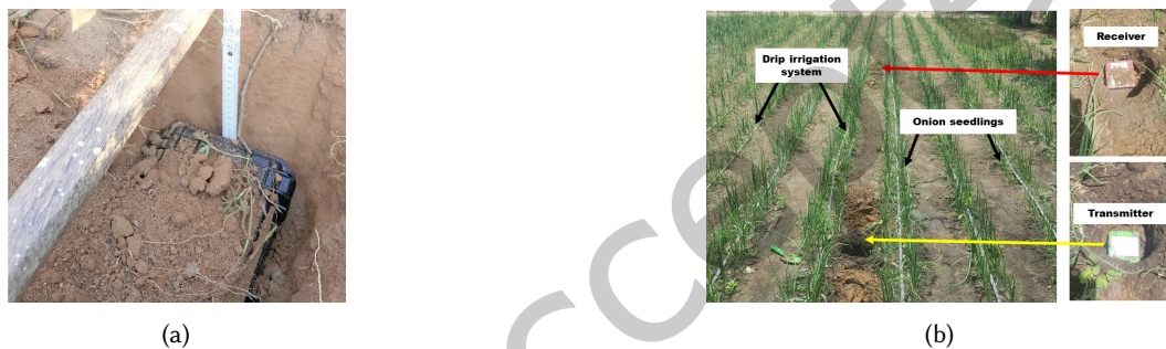
Fig. 3. Buried sensor nodes for ecological and agriculture monitoring. (a) Deployment of the MoleNet sensor node enclosed in a waterproof box in Ngaoundéré, Cameroon. (b) Application of a WUSN for onion culture within the Botanical Garden of the University Cheikh Anta Diop of Dakar in Senegal
