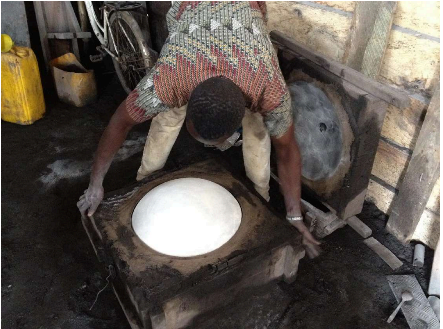
Fig. 7. Aluminium sand casting method. Credit: AMP.
