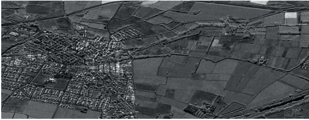
Figure 6 ONERA-DEMRA airborne measurement with the system SETHI over Sainte-Marie-la-Mer area at 0.5m resolution and 60° incidence angle.
