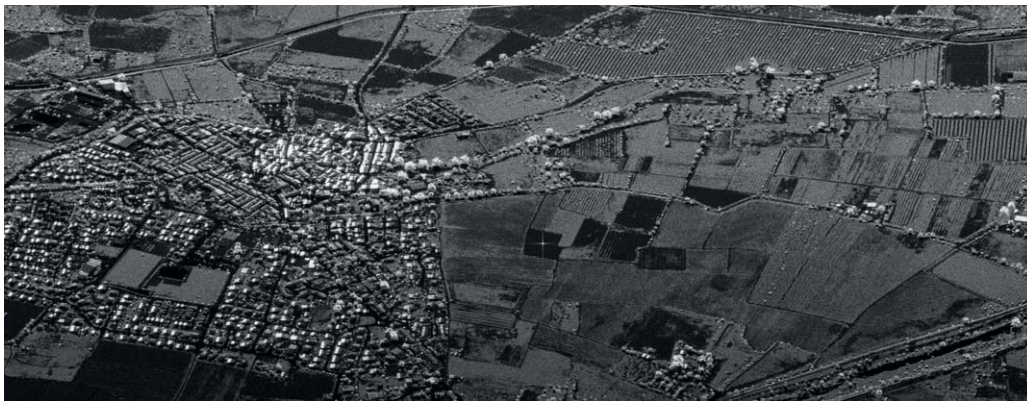
Figure 7 EMPRISE simulation of airborne SAR acquisition over Sainte-Marie-la-Mer area at 0.5m resolution and 60° incidence angle.
