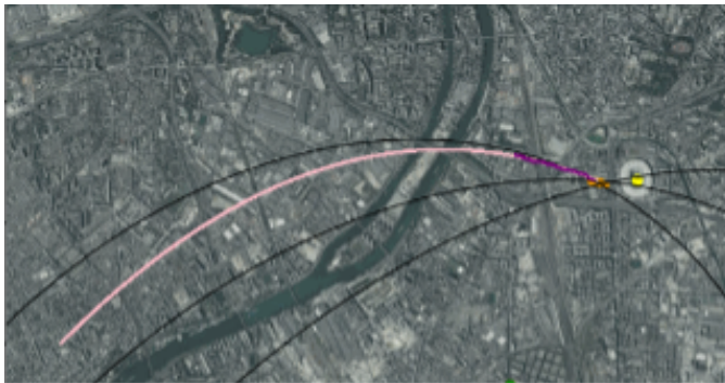
Fig. 6: Particle tracking filter simulation considering 1 target around the Stade de France . The black lines are potential considered trajectories, the pink line is the final chosen trajectory and the purple line is corresponding to the particle filter results. These simulations are processed with 2 receivers.
