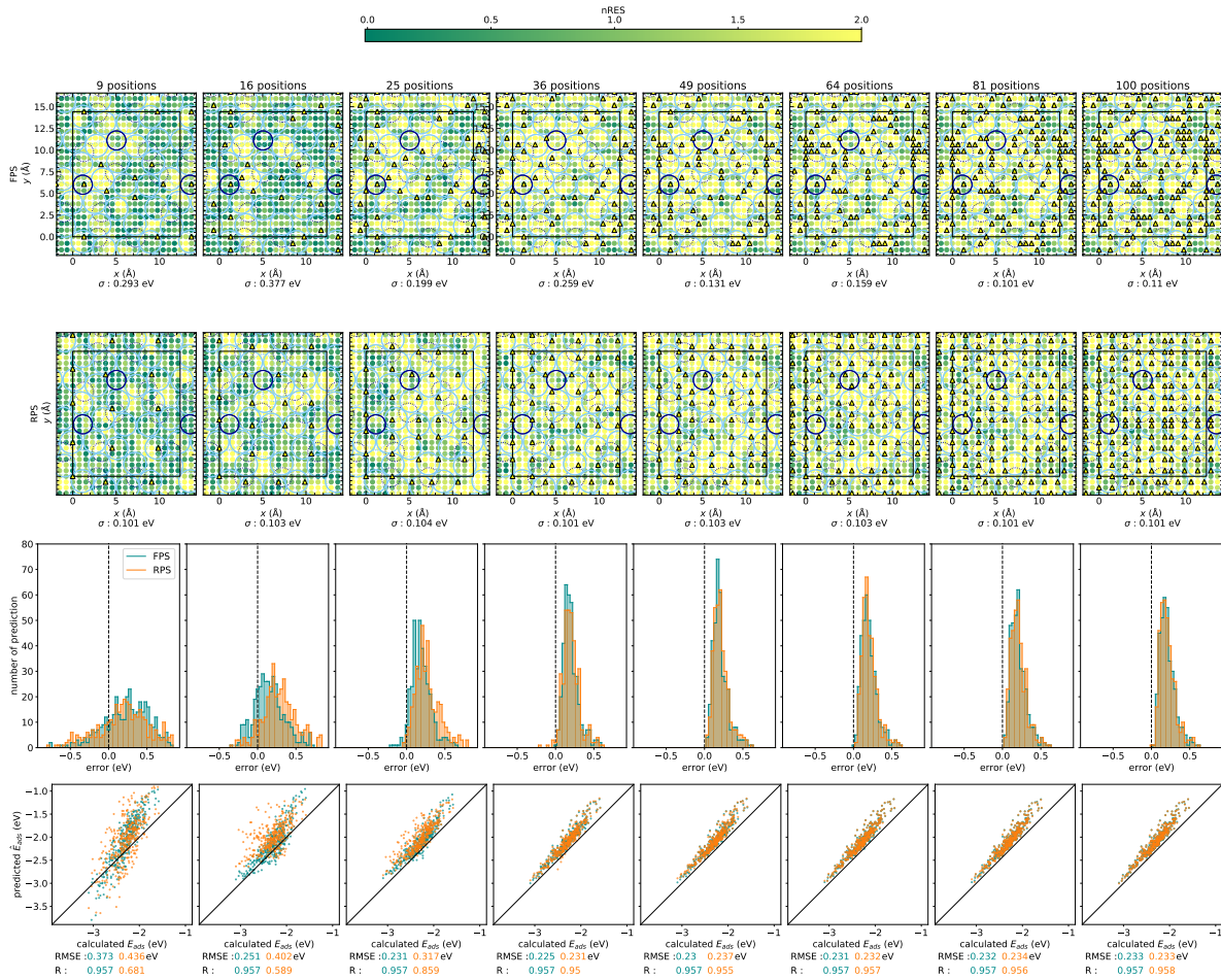
Figure S27: Error maps and histograms for atomic Lead adsorption energies. Training is done on E_{ads}^{nr} ( fixed ). Results are compared with E_{ads}^r ( relaxed ). The positions are selected on regular grids and FPS method.
